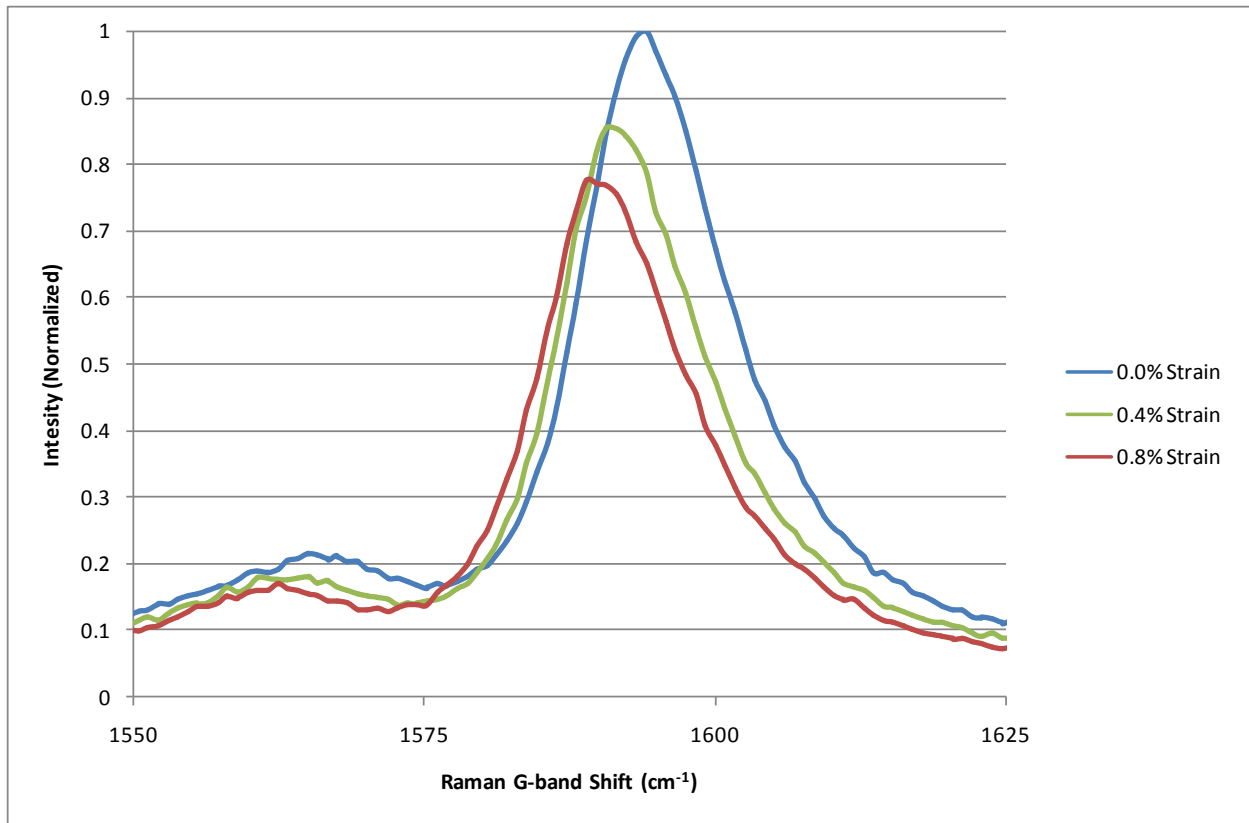
Figure 22: Raman spectra of the G-band for 0.25 wt % SWCNT composite at various tensile strains.
